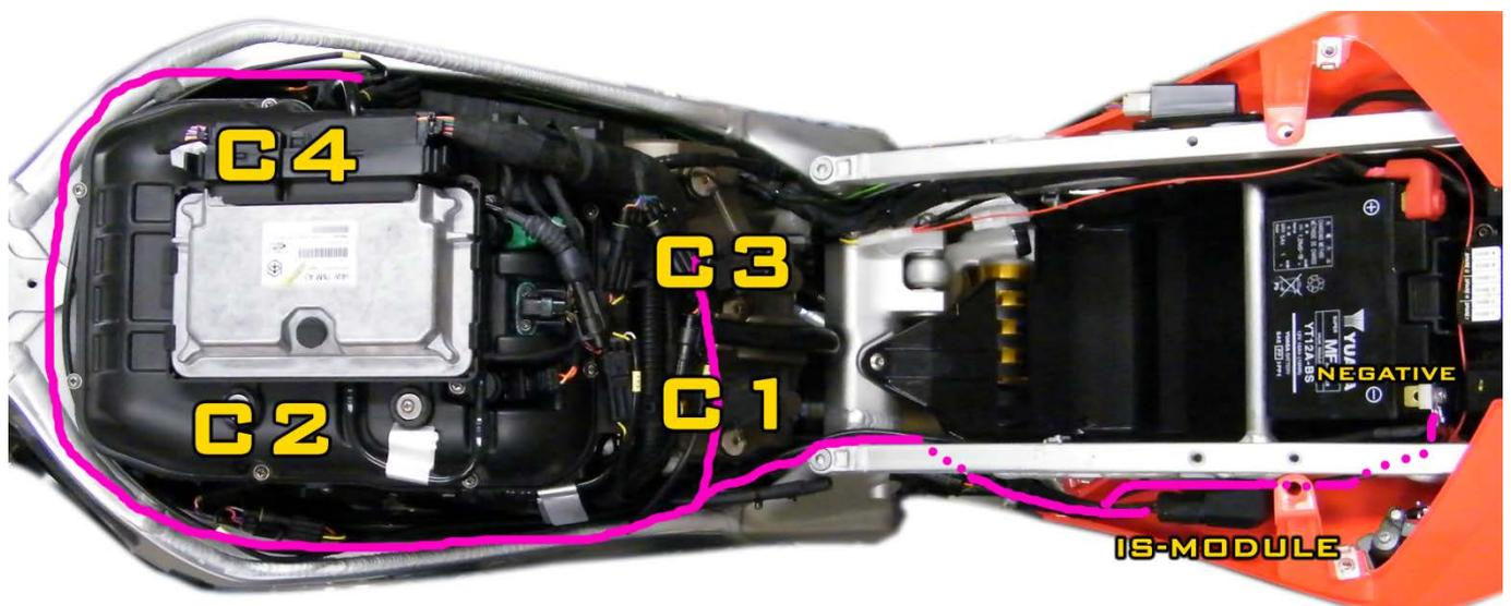
2. Connect the Power Shift connectors with those of the corresponding coils by following the label on the supplied cable and the position of every single cylinder, just as it is specified by the following images.
