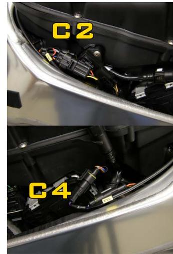
**Attention!: It is very important to connect the coil cables directly to avoid any damage; in particular, for cylinders 1 and 3 follow the wire of original connectors to find out the correct coil.**
