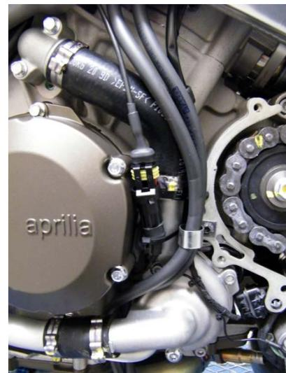
*At the end of the installation, it is recommended to secure the wiring by means of plastic clamps without pulling them too much to prevent them from damaging the wiring.*
