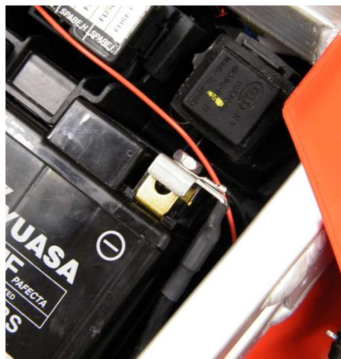
4. Use the supplied adhesive Dual Lock system to secure the IS-MODULE and the POWER SHIFT central unit, according to the figure, and connect them with the supplied wiring. It is important for the Power Shift central unit cable to run inside the saddle frame, according to the figure.
