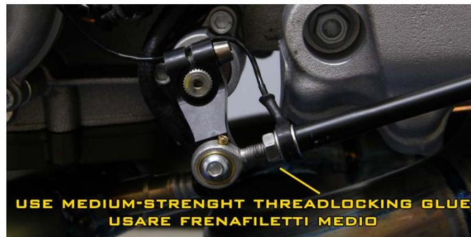
*Please Note: To prevent the lock nut from unscrewing as a result of vibrations, it is recommended to use medium-strength threadlocking glue on the uniball thread.*
